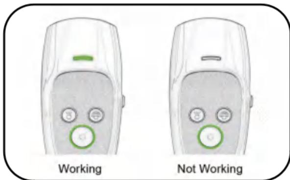
4. First, Try a test to make sure the green indicator light is ON when you press any button, which means the device is working perfectly. If the indicator light does not light up, please contact us at **support@nzonpet.com**. The professional customer service team will have a dedicated customer service staff to solve it.
