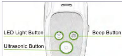
2. Light button: There are two ways to use it; a short press or a long press. It will emit a long bright light when short press, and a burst flashing when long press. The working status includes: the green indicator light is on and the bright LED light is on;
