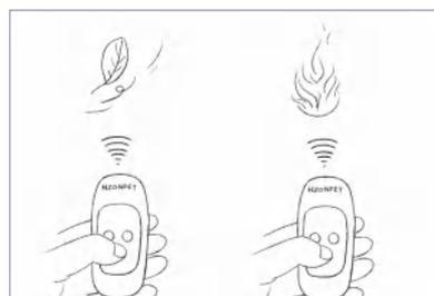
5. Testing the ultrasonic working status: Make sure the green indicator light is on when you press the ultrasonic button.
